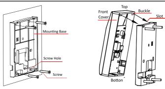
Figure 4-4 Install the Mounting Base
