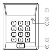
Figure 2-1 Appearance of Access Control Terminal
