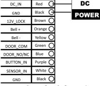
Figure 3-1 Power Supply Connection Diagram
