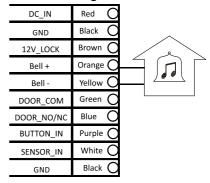
Figure 3-2 Doorbell Wiring Diagram
