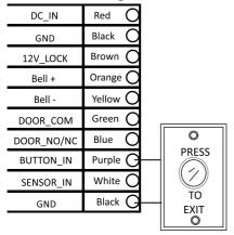
Figure 3-3 Door Button Wiring Diagram
