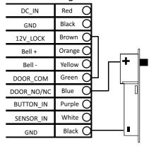
Figure 3-4 Door Lock Wiring Diagram
