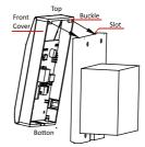
Figure 4-2 Attach the Front Cover
