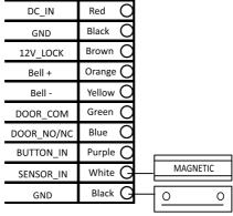
Figure 3-5 Door Magnetic Wiring Diagram
